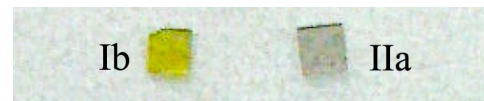
Fig. 2. Pristine single-crystals of IIa-type diamond (right) and Ib-type diamond (left, for comparison). The size of each crystal is approximately 1 \times 1 \times 0.3 mm 3 .
