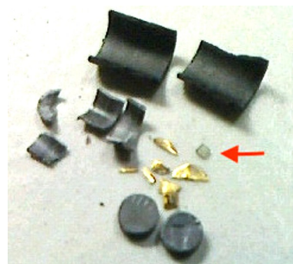
Fig. 3. The boron-implanted diamond (arrowhead) after the process of high-temperature and high-pressure annealing. Parts of high-pressure media are also shown.
