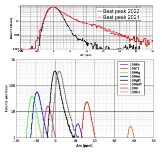
Fig. 1. (top) Comparison of MRTOF peak shape from 2021 with the improved peak shape achieved in 2022. (bottom) Simulated spectrum for A = 199 isobars based on measured MRTOF peak shape and calculated production yields. Prior to improving the peak shape it was very difficult to observe <sup>199</sup>Ir ions as they produced only a small fluctuation in the tail of the <sup>199</sup>Pt ion peak.
