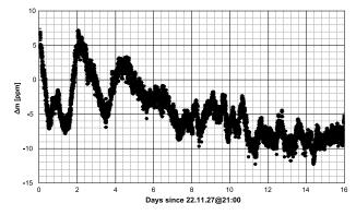
Fig. 2. Drift of the peak position over 16 days of measurement while roughly regulating the MRTOF chamber at 38°C. The maximum fluctuation is consistent with a thermal fluctuation of  $\Delta T_{pk-pk} \approx 0.75$  K.
