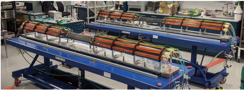
Fig. 5. Two INTT half barrels being assembled at BNL. In both of the half INTT, the B0L0 barrels are assembled.
