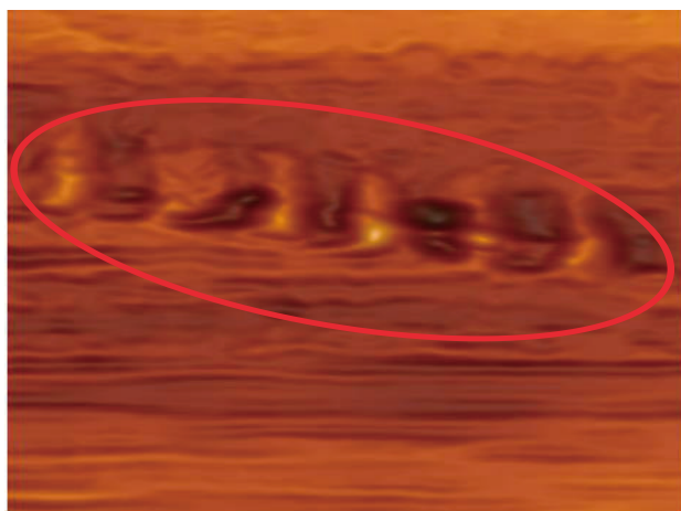
Fig. 1. STM image of 12 mer-dsDNA GC molecules aligned in one-dimensional chain structure.
