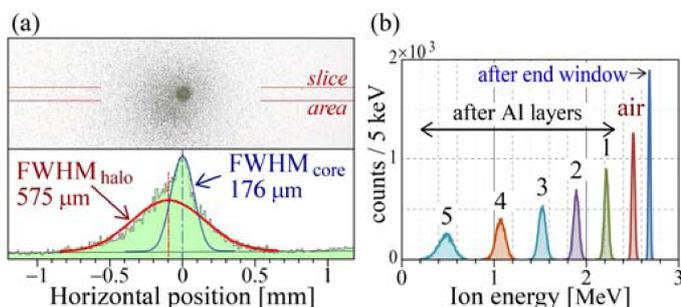
Fig. 1. (a) 2.8 MeV  $\text{H}^+$  microbeam spot on CR-39 and the histogram along with slice area. (b) Ion energies after transmitting the materials estimated by SRIM simulation. No ions were transmitted through more than five layers.
