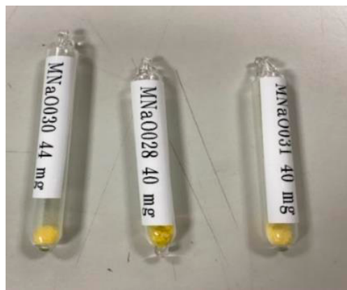
Fig. 1. Some sample batches of NaO 2 used for \mu SR experiment. Labels indicate the number of sample batches. Bright and dense yellow color imply that sample quality is good.
