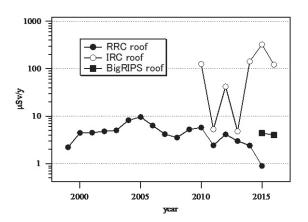
Fig. 1. Radiation dose at the boundary of the radiation-controlle area.
