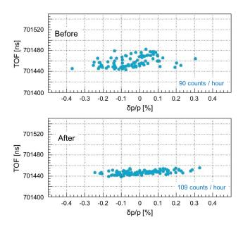
Fig. 2. TOF spectra of <sup>78</sup>Ge after extraction as a function of momentum. Upper and lower figures show the results obtained before and after adjusting the isochronism by the second order, respectively.
