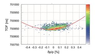
Fig. 1. TOF spectrum of <sup>78</sup>Kr after extraction as a function of momentum. The red line shows a quadratic fitting curve.
