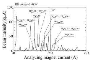
Fig. 2. Charge distribution of the highly charged Zn ion beam.
