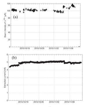
Fig. 1. (a) Beam intensity of  $U^{35+}$  ions and (b) the extracted current as a function of time.
