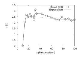
Fig. 2. Interaction cross sections of <sup>93</sup>Zr on <sup>12</sup>C. The results of the simulation (open circles with solid line) are shown with the expected values in PHITS (dotted-line).
