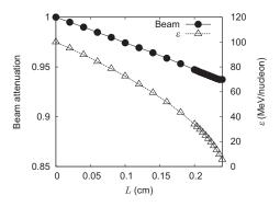
Fig. 1. The attenuation (solid circles with solid line) and energy (open triangles with dotted-line) of the incident beam are shown as a function of the target thickness.
