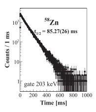
Fig. 1. Time correlations between  $^{58}$ Zn implanted ions in WAS3ABi and the 203 keV  $\gamma$  rays detected in EURICA.The solid line represents the fit to the decay curve
