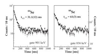
Fig. 2. Time correlations between  $^{64}{\rm Se}$  (left) and  $^{66}{\rm Se}$  (right) ions implanted in WAS3ABi and 901 and 836 keV  $\gamma$  rays respectively detected in EURICA. The solid lines represents the fit to the decay curves.
