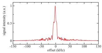
Fig. 2. NMR signals of the <sup>1</sup>H spins in flowing water in thermal equilibrium. Offset means the difference between the resonance frequency of <sup>1</sup>H and the frequency of electromagnetic waves.
