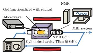
Pump (1.5 mL/min) Electromagnet (0.3 T)
