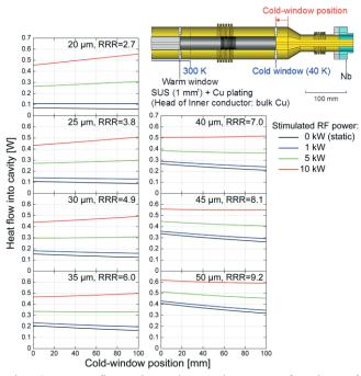
Fig. 2. Heat flows into the cavity as a function of cold-window position for various sets of thickness and RRR of copper plating. The configuration of the input coupler and the definition of cold-window position are also shown.
