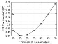
Fig. 3. Heat flows into the cavity for various thicknesses of copper plating (open circle) with realizable cold-window position. Stimulated RF power is 10 kW. As a reference, heat flows based on measured RRRs are also shown (filled square).
