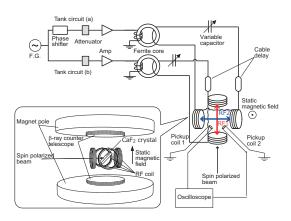
Fig. 1. Block diagram of the RF system for the rotating magnetic field and a schematic layout of the  $\beta$ -NMR setup.
