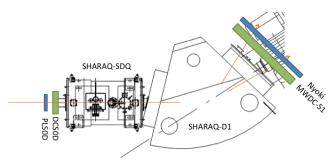
Fig. 1. Experimental setup before S1 focal plane of SHARAQ spectrometer.
