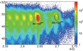
Fig. 1. Particle identification plot of the secondary beam after the liquid Helium target, gated on incoming <sup>132</sup>Sn ions determined using the ZeroDegree spectrometer.
