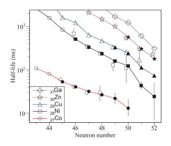
Fig. 1. Experimental half-lives as a function of neutron number for isotopes with Z = 27 - 31. All the solid symbols represent the half-lives determined in this work while the open symbols are the half-lives taken from the literature $^{1-4}$ . The systematic trends in the different isotopic chains are highlighted by lines connecting the data points with a smaller uncertainty.
