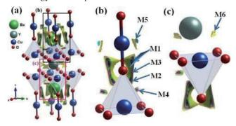
Figure 1. Crystal structure of YBCO with x=0. Cu(II) in the CuO<sub>2</sub> plane is surrounded by five oxygen atoms and has a spin half. The Cu(II) rules the antiferromagnetically ordered state, while the Cu(I) which is in the Cu-O chain is non-magnetic with a zero spin. We found six local minimum potential positions (M1 to M6) from the calculation by the DFT method. The positions were drawn by the isosurfaces in different colors.
