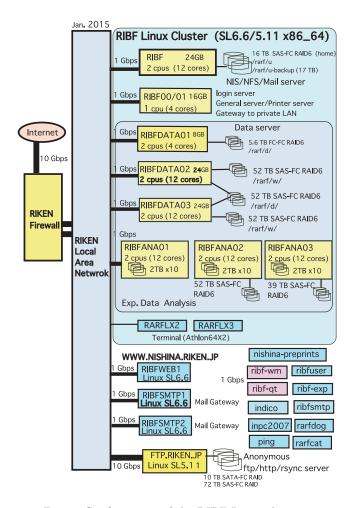
Fig. 1. Configuration of the RIBF Linux cluster.
