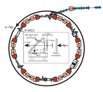
Fig. 1. Setup of  $\alpha$ -source and detectors. The carbon foil detector was placed in front of the  $\alpha$ -source, whereas the plastic scintillator was placed behind.
