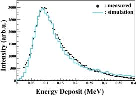
Fig. 2. Energy deposit distribution of the first layer for  $\beta$ -rays from the  $^{90}\mathrm{Sr}/^{90}\mathrm{Y}$  source.
