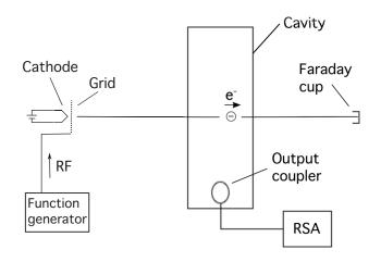
Fig. 1. Schematic view of the offline test using an electron beam. To induce an alternative electromagnetic field inside the resonant cavity, we use the grid to modulate the DC electron beam at the resonance frequency. Therefore alternative electromagnetic fields are induced by electrons passing through the resonant cavity. We detect the induced signals with a real time spectrum analyzer (RSA).
