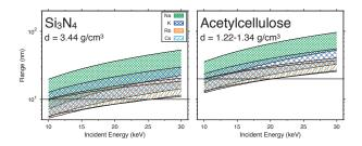
Fig. 2. Ranges as a function of the incident energy of an incoming ion beam for several elements with both SiN and Acetylcellulose membranes. The bands describe the range straggling in  $\pm 1\sigma$  and the dashed lines indicate the minimum thicknesses for each material.
