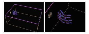
Fig. 2. Event display for a cosmic ray detected by the  $S\pi RIT$ -TPC in the SAMURAI magnet at 0.3 T. Enlarged view of the track is on the right.
