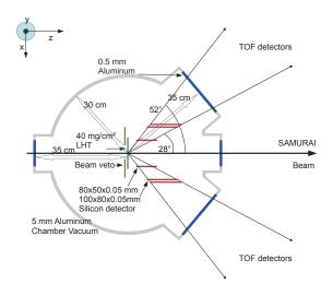
Fig. 1. Target chamber (top view) including three layers of one-dimensional silicon strip detectors on each side.
