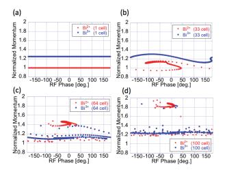
Fig. 2. Result of longitudinal phase space distribution. Red: Bi<sup>2+</sup>, Blue: Bi<sup>3+</sup>. The ordinate axis shows momentum normalized to Bi<sup>2+</sup> initial momentum. The abscissa shows RF phase. (a) Initial distribution, (b) after pre-bunching, (c) after capturing Bi<sup>2+</sup>, (d) after acceleration.
