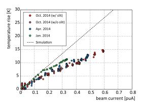
Fig. 2. Dependence of the temperature rise of helium on the beam current. Dotted line indicates the calculated values.
