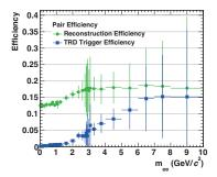
Fig. 1. p<sub>T</sub> integrated pair efficiency as a function of invariant mass. Circles and boxes correspond to the pair reconstruction efficiency and TRD trigger efficiency for pairs, respectively.
