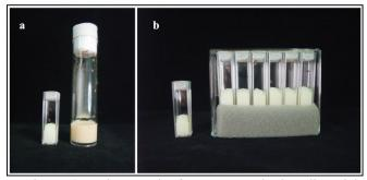
Fig. 1. a) A photograph of a cuvette and a breeding vial. b) A photograph of sample cuvettes for irradiation using an automatic sample changer.
