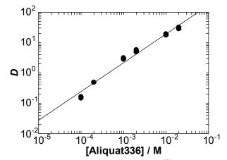
Fig. 1. Variation of the distribution ratio of  $^{181}$ W from 1.0 ×  $10^{-2}$  M oxalic acid with 0.1 M HCl/0.9 M LiCl as a function of the concentration of Aliquat 336.
