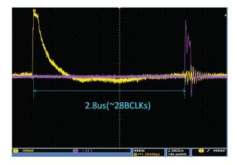
Fig.2 Coincidence between calibration pulse (yellow) and trigger signal (pink)
