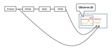
Fig.1 Setup of the timing measurement using a scope and FVTX readout devices  $^{1)}$
