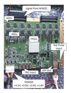
Fig. 1. View of 64ch Readout Board.
