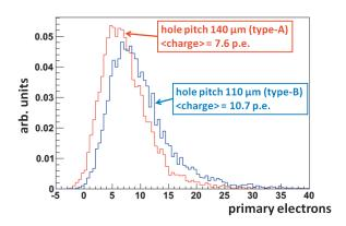
Fig. 2. Charge distribution of two different photocathodes.
