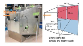
Fig. 1. Photograph (left) and schematic view (right) of the HBD prototype.
