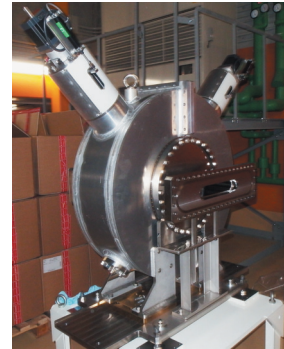
Fig. 1. The resonant Schottky pick-up that will be installed in the Rare-RI Ring. The resonant cavity surrounds the beam pipe with a ceramic gap. The lower flanges for feedthroughs are the output coupler loop, and the upper feedthroughs are the movable plunger pistons, using which the resonance frequency of the eigenmode can be adjusted.
