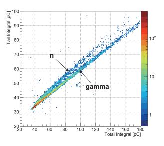
Fig. 2. Pulse shape discrimination between neutrons and gamma rays in EJ299-33.
