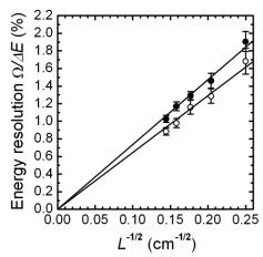
Fig. 1. Dependence of energy resolution on gas thickness obtained for heavy ions Z=38 (solid circles) and Z=51 (open circles). The solid lines are the results of linear fitting, which show the linear dependence on  $L^{-1/2}$ .
