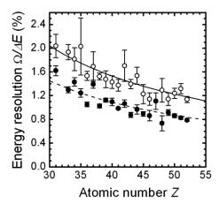
Fig. 2. Energy resolution as a function of the atomic number of fragment heavy ions produced from the in-flight fission of <sup>238</sup>U at 345 MeV/nucleon. Open and solid circles represent the cases with L=24 cm and L=48 cm, respectively. The solid and dotted lines are the results of the fitting of  $Z^{1}$ .
