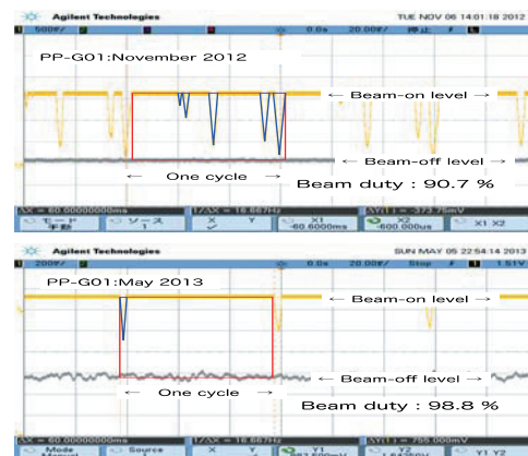
Fig. 3. Signals of phase probe monitor (PP-G01). Vertical axis: beam intensity. Horizontal: scan time.
