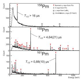
Fig. 1. Preliminary  $\gamma\text{-ray energy spectra of <math display="inline">^{158}\mathrm{Pm},~^{159}\mathrm{Pm}$ and  $^{161}\mathrm{Pm}.$  The time windows of  $^{158}\mathrm{Pm}$  is up to  $16\mu\mathrm{s}$ and that of  $^{159}\mathrm{Pm}$  and  $^{161}\mathrm{Pm}$  are up to  $5\mu\mathrm{s}.$  Events close to the timing of the beam implantation are excluded. Half-lives of  $^{159}$ Pm and  $^{161}$ Pm are obtained from the 330 and 728 keV  $\gamma$  ray respectively.
